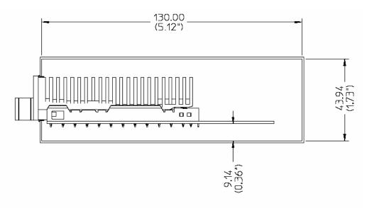
Figure 16 Cross Section of Test Fixture
