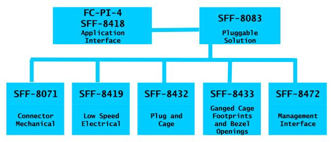
FIGURE 3-1 SPECIFICATIONS NEEDED TO IMPLEMENT A 10 GB/S PLUGGABLE TRANSCEIVER
