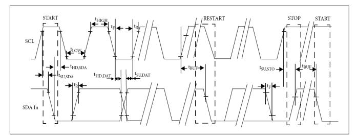
FIGURE 12 2-WIRE TIMING DIAGRAM
