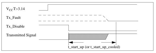
FIGURE 5 POWER ON INITIALIZATION OF MODULE, TX\_DISABLE ASSERTED
