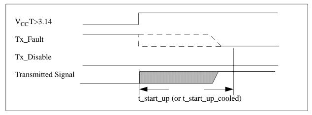
FIGURE 6 EXAMPLE OF INITIALIZATION DURING HOT PLUGGING, TX\_DISABLE NEGATED
