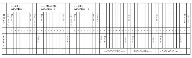
FIGURE 17 SEQUENTIAL ADDRESS READ STARTING WITH RANDOM READ
