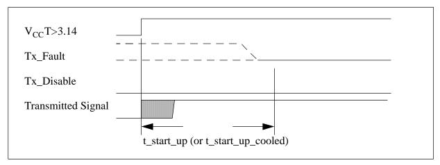
FIGURE 4 POWER ON INITIALIZATION OF MODULE, TX\_DISABLE NEGATED
