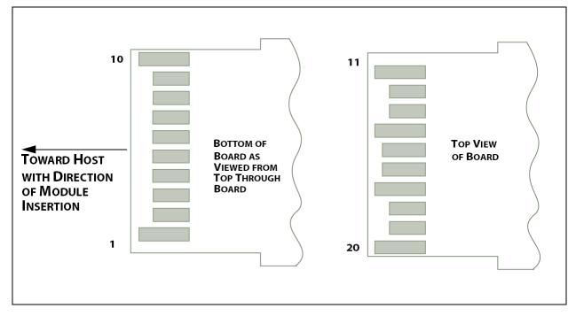
FIGURE 3 SFP+ MODULE CONTACT ASSIGNMENT
