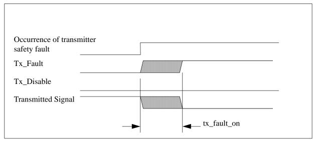
FIGURE 8 OCCURRENCE OF CONDITION GENERATING TX\_FAULT
