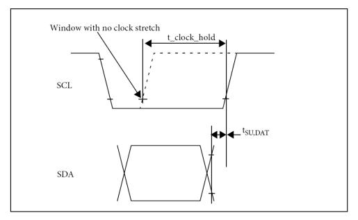
FIGURE 13 DETAIL OF CLOCK STRETCHING
