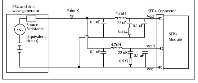
FIGURE 22 POWER SUPPLY NOISE TOLERANCE TEST SETUP
