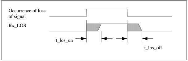
FIGURE 11 TIMING OF RX\_LOS DETECTION
