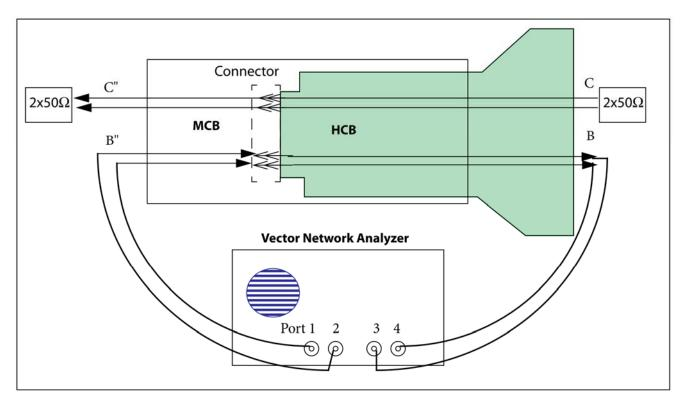
FIGURE 3 MCB-HCB S-PARAMETERS TEST SETUP
