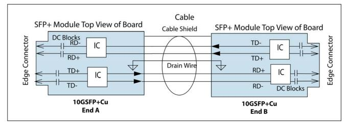
FIGURE 1 10GSFP+ACA DIRECT ATTACH BLOCK DIAGRAM
