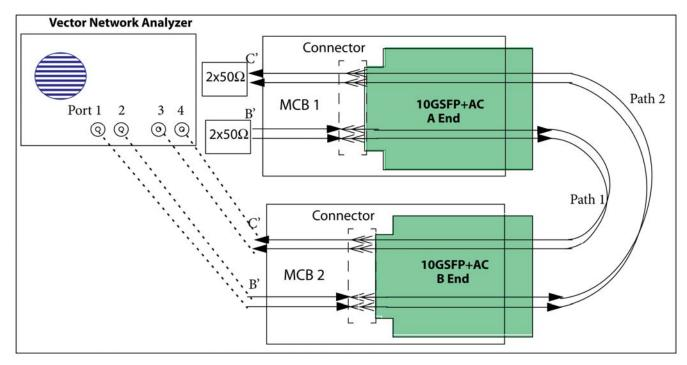
FIGURE 5 CABLE S-PARAMETERS CROSSTALK MEASUREMENT
