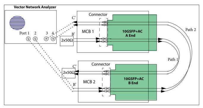
FIGURE 4 CABLE S-PARAMETERS THROUGH TEST SETUP
