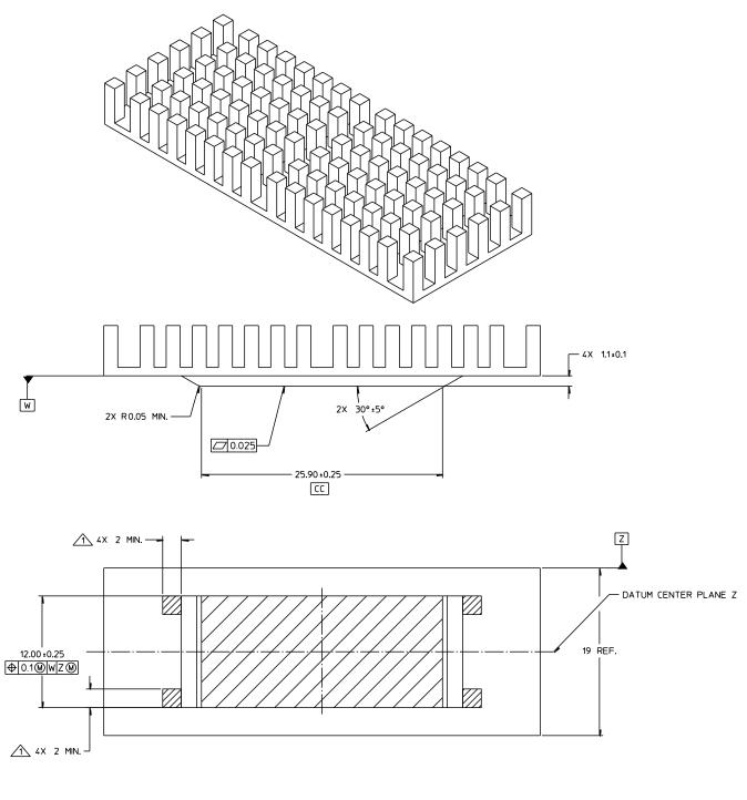
1 PLANE FOR FLATNESS AND HEIGHT MEASUREMENTS ESTABLISHED AT FOUR INDICATED AREAS 2. ALL OTHER DIMENSIONS ARE PER MANUFACTURER DESIGN
