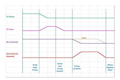
FIGURE: 7-1 CHANNEL TO CHANNEL SWITCHING IN LOW POWER MODE
