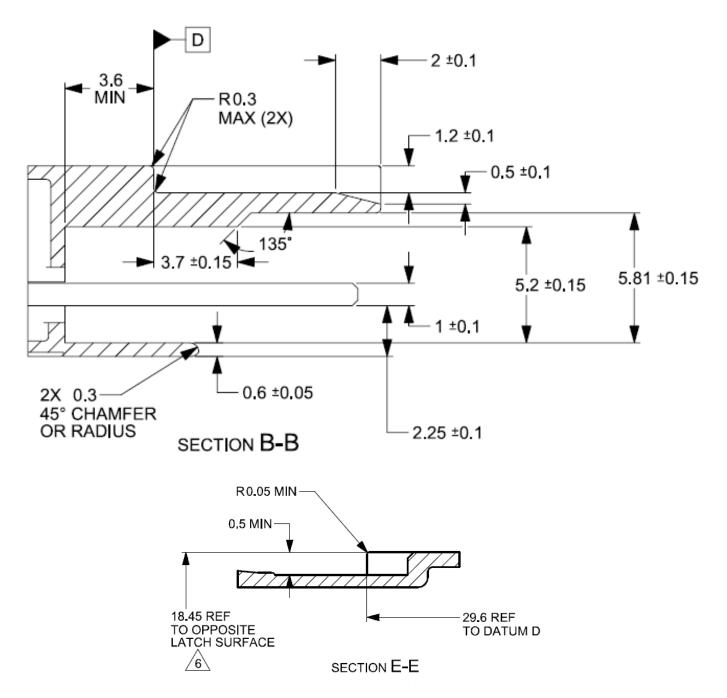
Figure 20: Detailed dimensions of module
