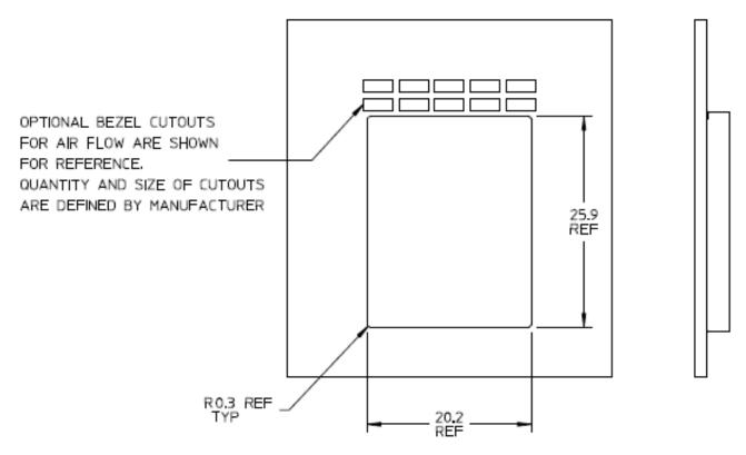
Figure B-3: Type 2A example 2X1 bezel design
