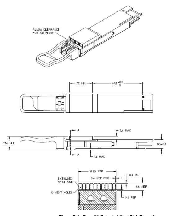
Figure B-4: Type 2A Extruded Heat Sink Example
