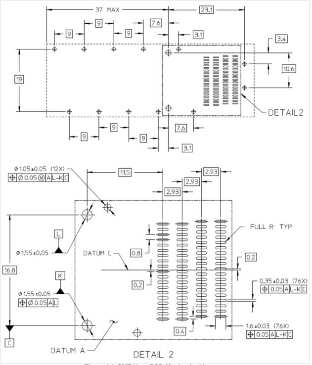
Figure 34: SMT Host PCB Mechanical Layout
