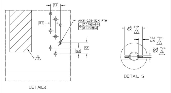
Figure 29: 2X1 Host PCB Mechanical Layout
