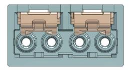
Figure 41: Dual CS connector module receptacle (in support of breakout applications)
