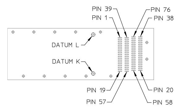
Figure 35: SMT Connector and Host PCB Pin Numbers
