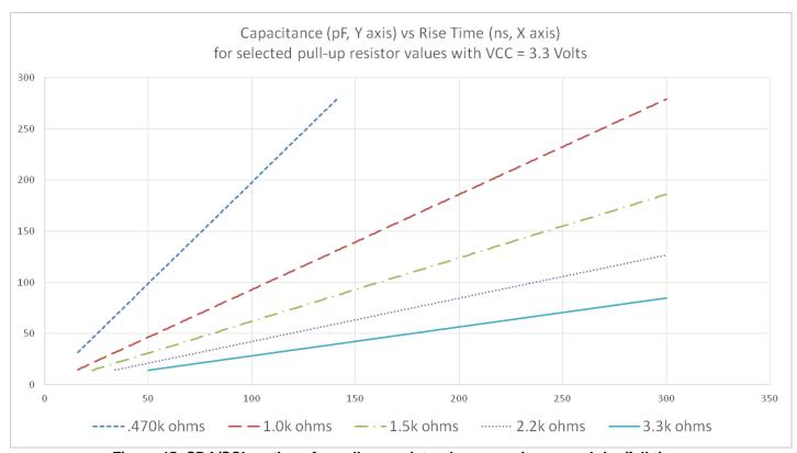
Figure 45: SDA/SCL options for pull-up resistor, bus capacitance and rise/fall times
