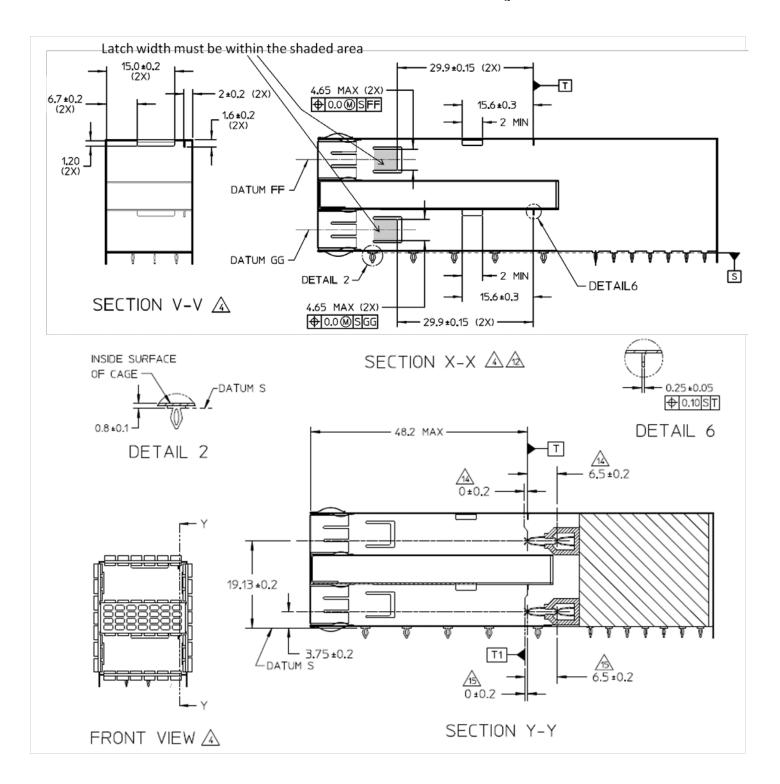
Figure 25: 2x1 stacked cage dimensions
