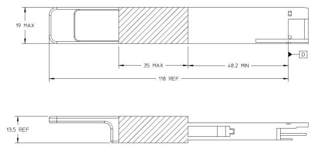
Figure 47: Informative overall module length with handle for Type 2 and Type 2A modules
