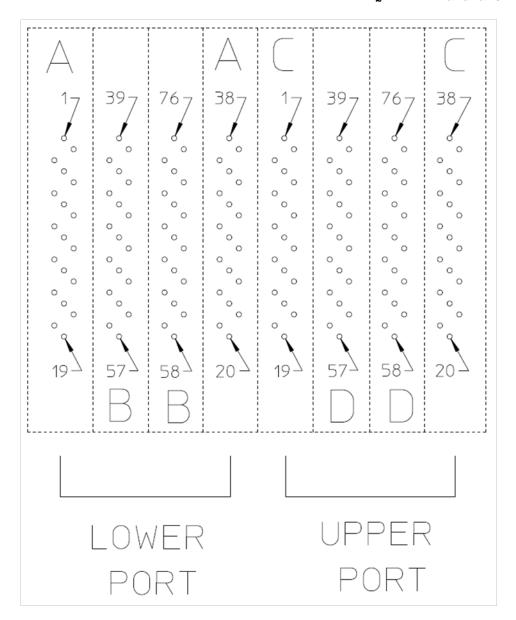
Figure 28: 2X1 host board connector contacts
