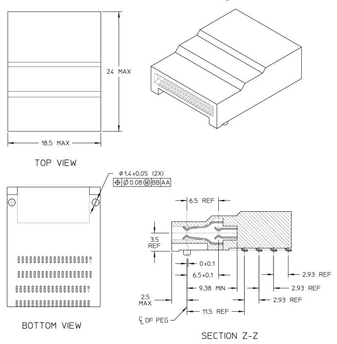
Figure 32: SMT 1x1 Connector Design
