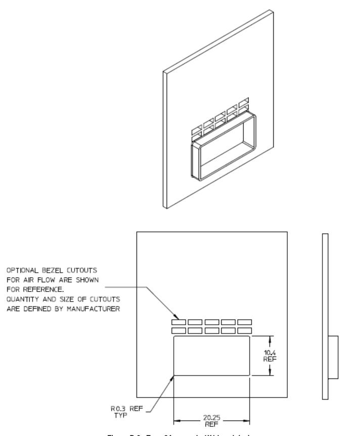
Figure B-2: Type 2A example 1X1 bezel design
