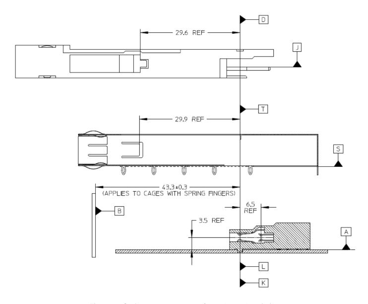
Figure 14: Surface mount connector/cage datum descriptions
