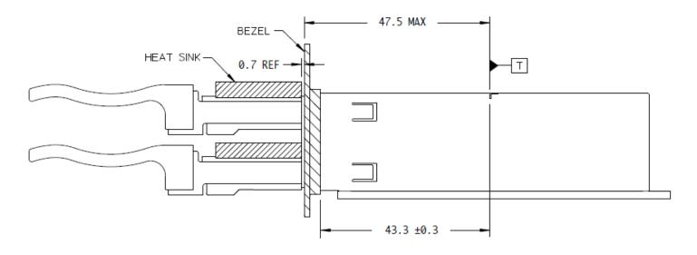
Figure B-1: Type 2A example module insertion
