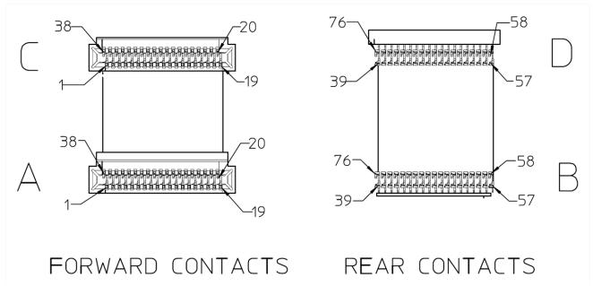
Figure 26: Connector pins in 2x1 stacked cage as viewed from the front
