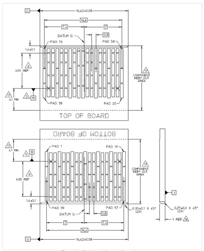
Figure 21: Module paddle card dimensions
