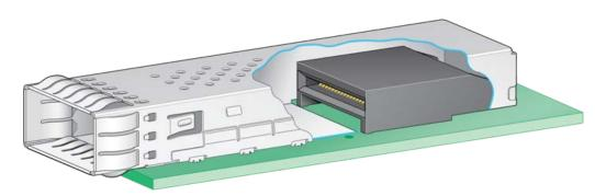
Figure 30: SMT connector in 1xn cage
