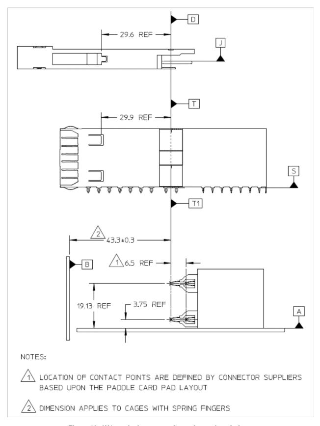
Figure 13: 2X1 stacked connector/cage datum descriptions
