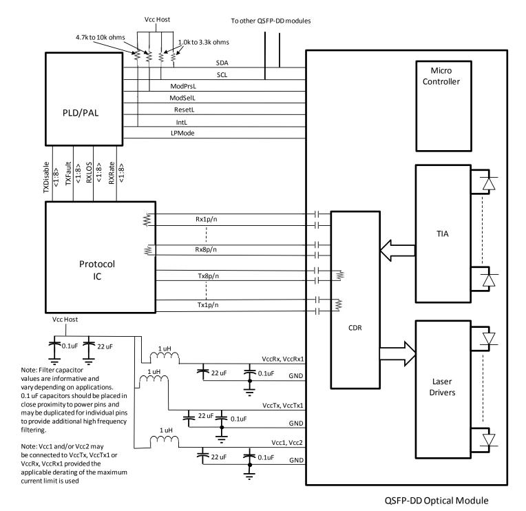
Figure 3: Example QSFP-DD Host Board Schematic For Optical Modules
