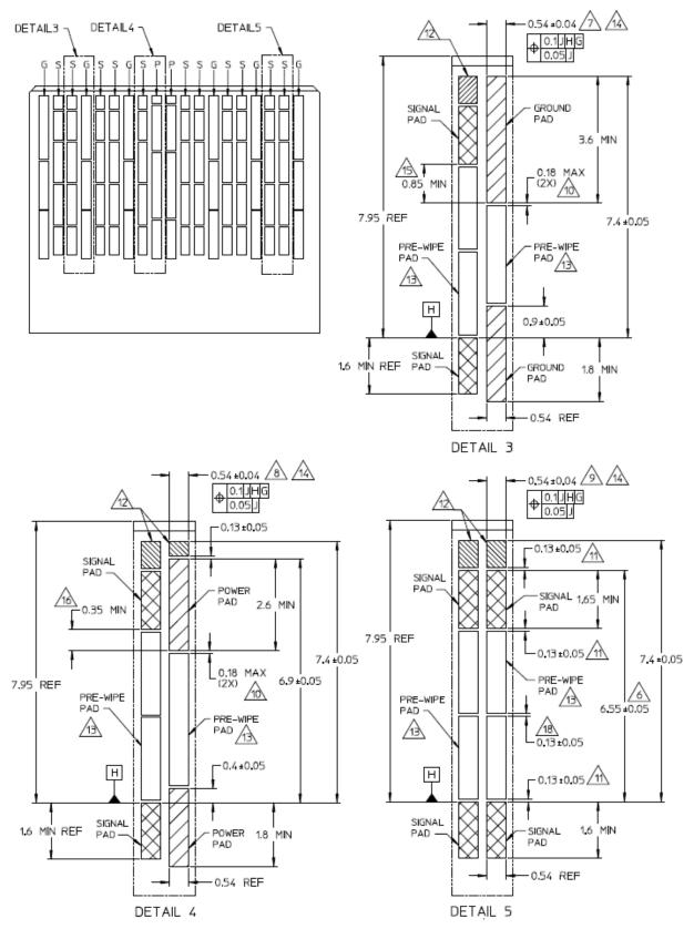
Figure 22: Module pad dimensions
